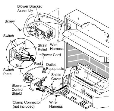
Figure 18 - Installing Blower Bracket Assembly
